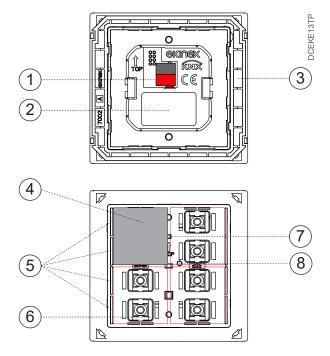
1) Connection terminal block for KNX bus line
