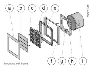
a)1-fold square plate, with a 60 x 60 mm window b)Rockers
