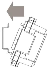
To mount the device, insert the mounting support into the appropriate shaped profile of the interface, then hook the teeth to the profiled guide starting from the bottom. Finally, push the upper part towards the guide for final coupling.
