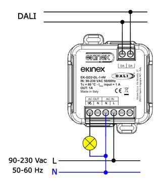
Three-wire connection diagram with common neutral
