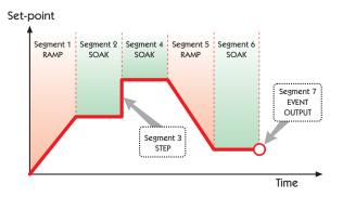
The CAL 9500P is potentially **the most versatile and flexible controller** in its size and price range. The program below shows what is possible from this unique controller.
