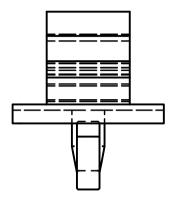
To Fit Panel Hole Ø4.8 Panel Thickness 1.8-2.8 mm
