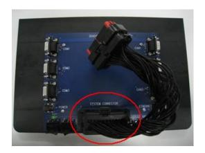
3. Connect the power cable to the Breakout Board.
