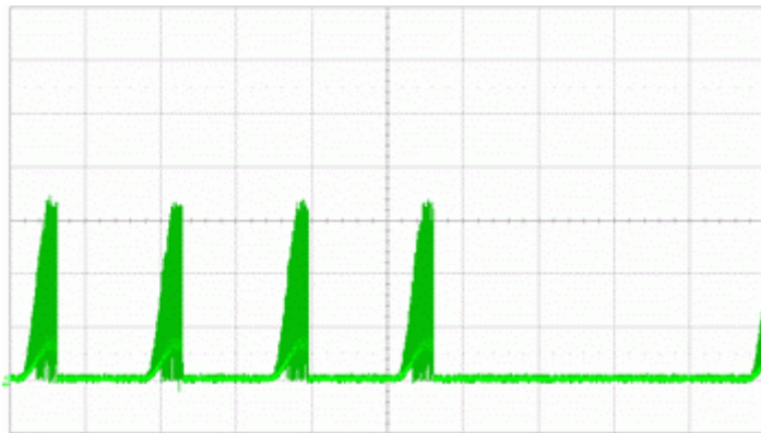
Blockierstrom @ 48 V ( I = 500\text{mA/div} ; t = 10\text{s/div} )
