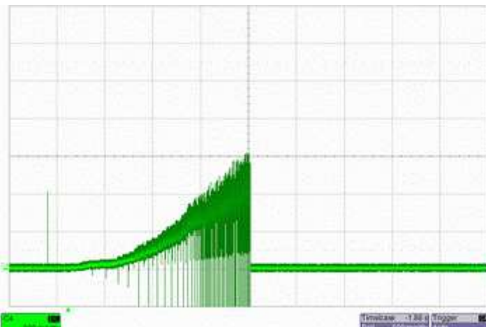
Blockierstrom @ 36 V (I = 500mA/div ; t = 500ms/div)
