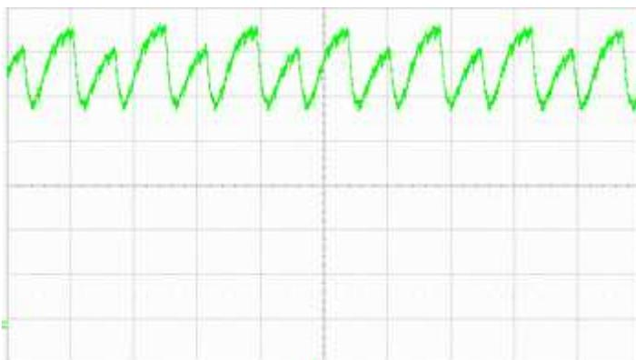
Laufstrom @ 24 V ( $I = 1\text{A/div}$  ;  $t = 500\mu\text{s/div}$ )
