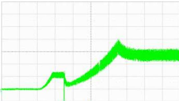
Anlaufstrom @ 24 V ( $I = 2\text{A/div}$  ;  $t = 2\text{s/div}$ )
