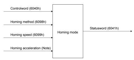
Note. In the point table mode, use the acceleration time constant and deceleration time constant in point table No. 1 (2801h).
