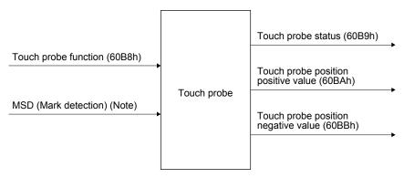
Note. Input with an external signal.
