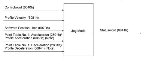
Note. For the point table method ([Pr. PA01] = \_ \_ \_ 6), set the acceleration time constant to Point Table No. 1: Acceleration (2801h), and the deceleration time constant to Point Table No. 1: Deceleration (2801h).
